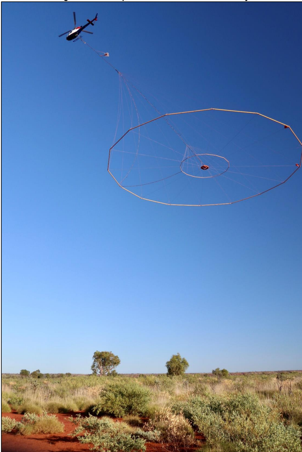
Figure 3 – Helicopter Assisted VTEM MAX Survey
